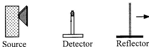
The waves reflected from the metal reflector plate interfere with the incident waves from the source. As the reflector is moved away from the detector, a series of maxima and minima are recorded by the detector.
