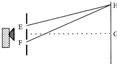
E and F are two slits in a metal plate. A microwave detector is moved along the line GH. H is the second minimum from the straight through point at G. (This is sometimes called the first-order ( $n = 1$ ) minimum, the first minimum being the zero order  $n = 0$ ) Measurement of distances EH and FH gives:  $EH = 0.421$  m and  $FH = 0.466$  m.
