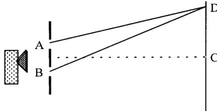
A microwave detector is moved along the line from C to D. The zero-order maximum of radiation is detected at C and the first-order maximum is detected at D.  $AD = 0.52$  m and  $BD = 0.55$  m.
